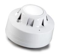
of 33 volts DC and a minimum of 9 volts DC in normal operation. The supply may fall to 6 volts DC in alarm conditions if a supply current of at least 10 mA is available at this voltage. To ensure effective illumination of the integral LED and any remote indicator, the supply to the detector should exceed 10 volts. To restore the detector to quiescent condition. necessary to expel any smoke and interrupt the electrical supply to the detector for a minimum of one second.
