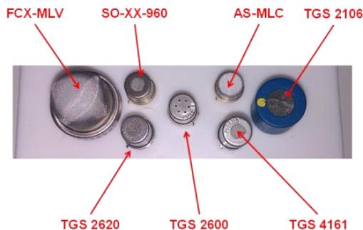
Fig. 1. Initial gas sensor array
